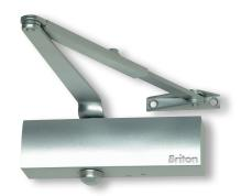
The Briton 200 Series is a compact door closer designed for use on residential or light commercial interior hollow core wooden doors e.g. electrical cupboards, storeroom and office doors. The 200 Series is not recommended for use on exterior door applications. For exterior door applications refer to the Briton 1120 and 1130 Series.
